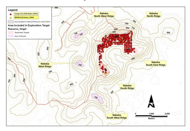
FIGURE 4: DRILLHOLE LOCATION PLAN, NABEBA DEPOSIT
