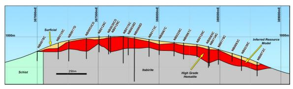
FIGURE 5: OBLIQUE SECTION THROUGH NABEBA LOOKING NORTH WEST SHOWING THICKNESS OF UP TO 144M OF HIGH GRADE HEMATITE)
