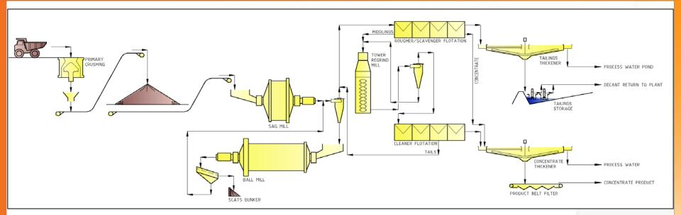
Proven grind and float beneficiation to produce concentrate; ~47% weight recovery
