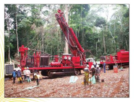
FIGURE 1 - RC DRILLING AT THE MBALAM ITON ORE PROJECT, CAMEROON (MARCH 2008)
